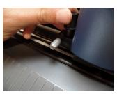
Remove the blade holder from the machine.
