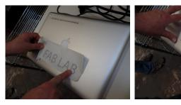
Apply it on the desired surface, carefully peeling off the masking tape.
