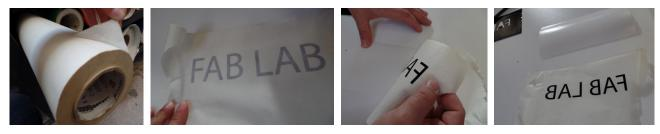
Cover it with the masking tape, avoiding any bubbles.
