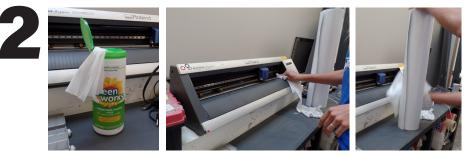
Wipe the dust off the machine, the space behind it, and the vinyl, using the cleaning wipes.
