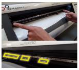
The rollers have to be placed within the white areas for the measurements to be accurate.
